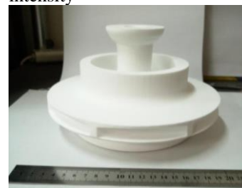
Figure 6. The flawless SLS prototype
