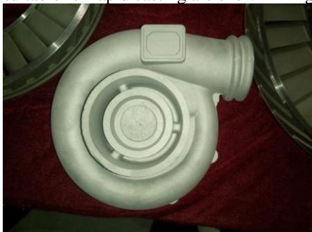
Figure 1. Castings suitable for rapid casting 3D Printing Technology includes Stereo Lithography Apparatus (SL), Selective Laser Sintering (SLS), Fused Deposition Modeling (FDM), Laminated Object Manufacturing (LOM) and 3Dimensional Printing (3DP). The parts manufactured by these printing methods have different applications because of different raw materials and working principles. SLA is based on liquid photosensitive resin as raw
