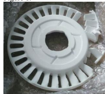
Figure 5. Prototype with defect due to insufficient intensity
