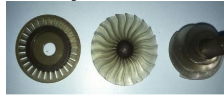
Figure 3. The part prototype made by mask projection technolog
